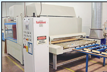
CEFLA/FALCIONI Kleenglass Horizontal Glass Spraying Machine, w/mixing system.
