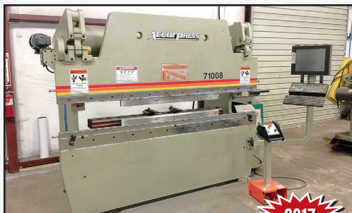
2017 ACCURPRESS CNC PRESS BRAKE , Mdl. 71008, s/n 12734, 100-ton x 8' O.A., Accurpress ETS3000 CNC controls and back gauge.
