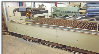
1998 MITSUBISHI LXP 3015 2D CNC LASER SYSTEM , s/n 6730LXP120, 2,000-watt, dual pallet shuttle tables, chiller w/pallet storage system.
